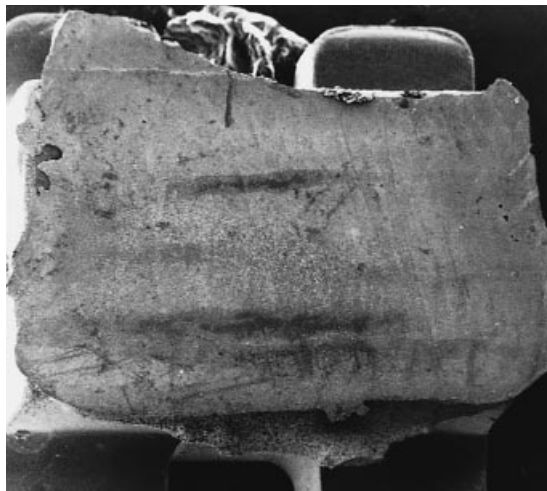
Figure 9 SEM of a Fascination/Dyract Ortho combination that debonded at the enamel-adhesive interface, showing the majority of adhesive on the bracket base ( \times 20.5 ).
