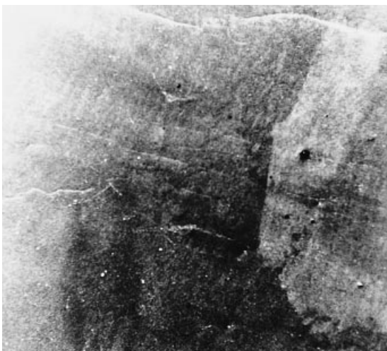
Figure 10 SEM of the enamel surface of a Fascination/Fuji Ortho LC combination which debonded at the enamel-adhesive interface, with more than 90 per cent of the bonded enamel free of adhesive ( \times 20.5 ).
